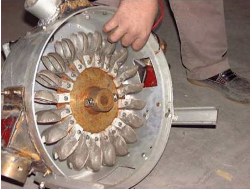
Fig. 3: Turbina Pelton (SOLENER)
